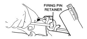
3 Test safety to see that it works in both positions. Weapon must not fire in S (safe).
